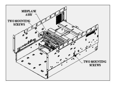
Figure 2-11: Midplane Assembly Installed in System
